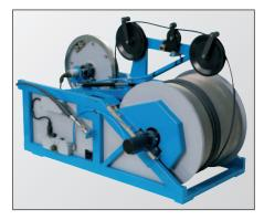
Winches: Robertson Geo designs and builds its own range of winches of varying capacities for deploying subsurface probes on 4-core or co-axial cable.
